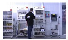
We have test stands developed by us, thanks to which we check whether the device is operational. They make sure that ALLEN BRADLEY 1398-PDM-020 is repaired.
